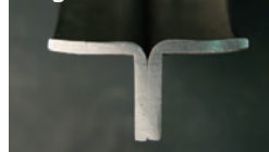
Cross section of stamped rings back to back
