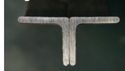
Cross section of rolled rings back to back
